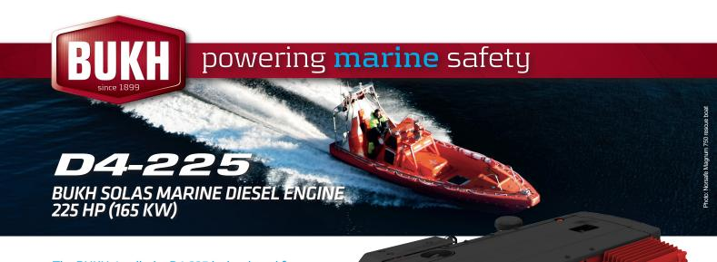
The BUKH 4-cylinder D4-225 is developed from the latest design in modern diesel technology. The engine has common rail fuel injection system, double overhead camshafts, 4 valves per cylinder, turbocharger and aftercooler.
