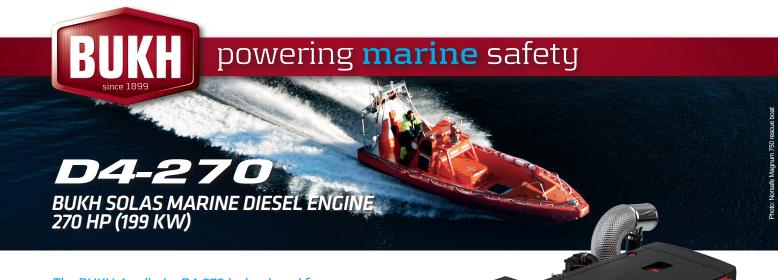
The BUKH 4-cylinder D4-270 is developed from he latest design in modern diesel technology. The engine has common rail fuel injection system, double overhead camshafts, 4 valves per cylinder, turbocharger and aftercooler.
