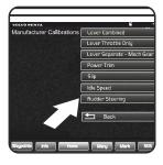
**5.** Manufacturer Calibrations > Rudder Steering.
