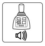
5. Buzzer and light confirm start of calibration.
