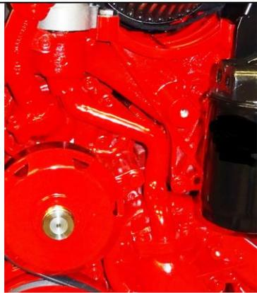
To install a water heater or cabin heater you must purchase the optional water heater tube available from BUKH. This will replace the original bypass tube installed on the engine.
